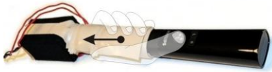
figure 1. Modified uWand. The arrow shows the direction of the haptic feedback as perceived by the user.
